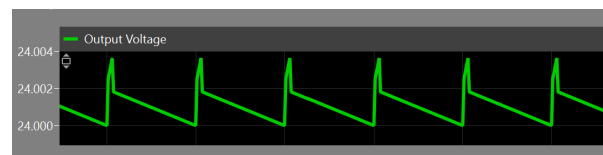
Output voltage stability between 6 and 7s
