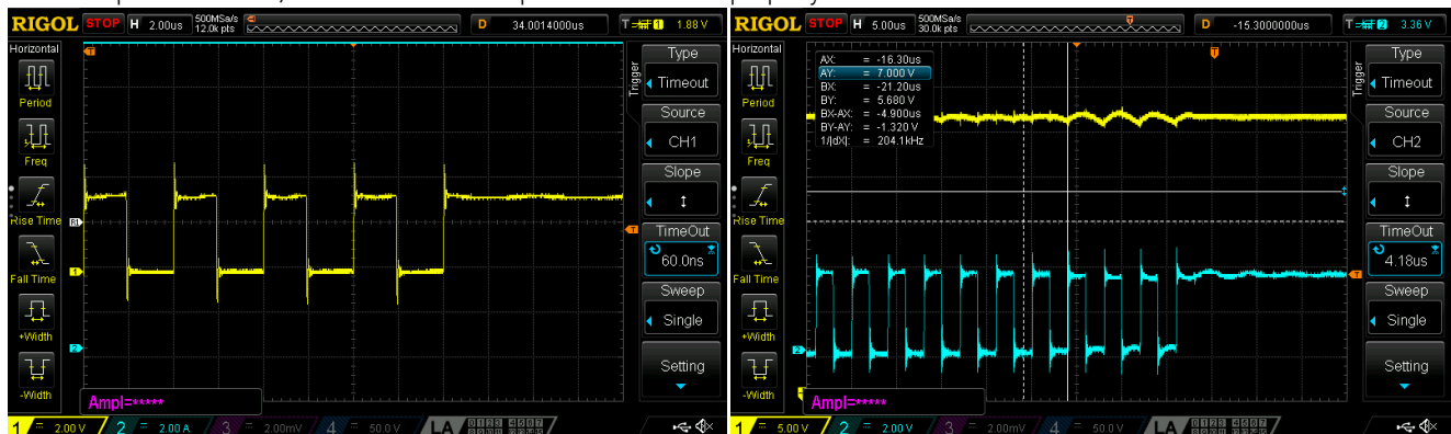
Picture 1: PWM1A during overvoltage detection.
