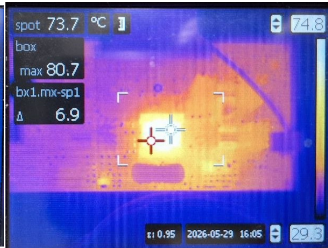
Picture 2: Thermal picture of the PCB after 10 minutes of test (Angle 2)
