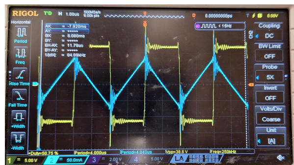
Figure 21 Secondary voltage with 24V in the secondary
