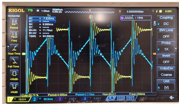
Figure 20 Primary voltage with 24V in the secondary
